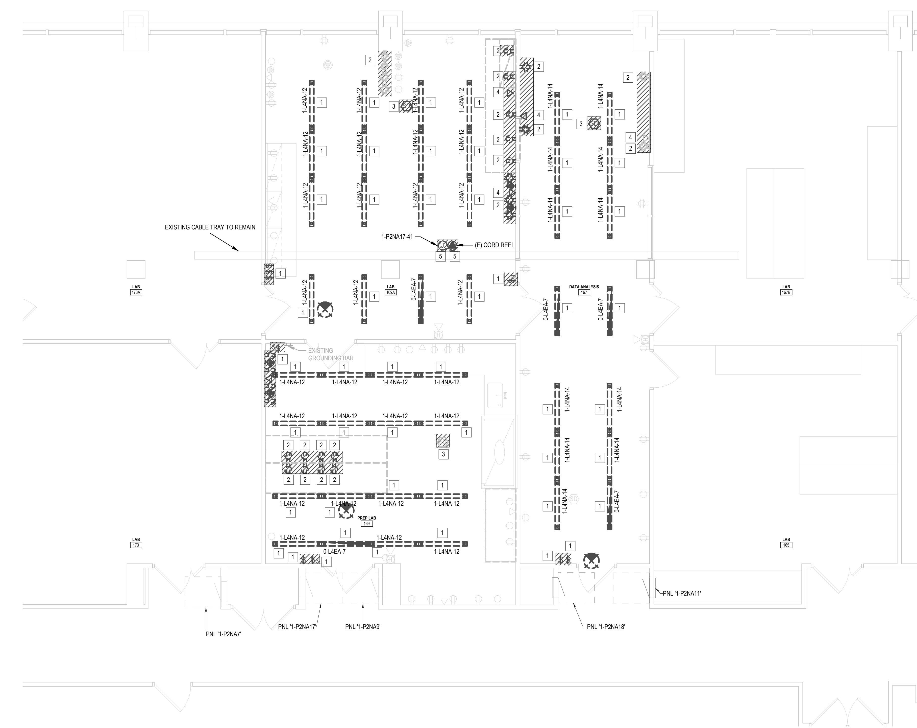
1 FIRST FLOOR ELECTRICAL PLAN - DEMOLITION SCALE: 1/4" = 1'-0"
