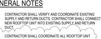
CONTRACTOR SHALL VERIFY AND COORDINATE EXISTING SUPPLY AND RETURN DUCTS. CONTRACTOR SHALL CONNECT NEW ROOFTOP UNIT INTO EXISTING SUPPLY AND RETURN
